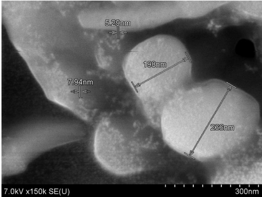
Figure 3 – SEM image of the morphology features of sorption materials of the composition MgO: FeZnOF at a concentration of (1:1) in moles, annealing in air at T=700 °C for 1 hour.
