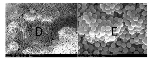
Photo FSEM ( D and E ) of Crosslinked PMMA nanoparticles
