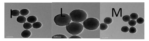
Photo (I,L and M) TEM of Crosslinked PMMA nanoparticles
