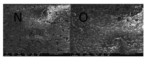
Photo (N and O) FSEM of Membrane of PMMA & PMMA crosslinked treated THF
