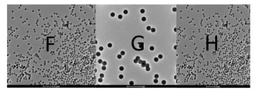
Photo (F,G and H) TEM of PMMA nanoparticles
